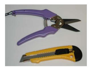
Fit each mat into place and make necessary cuts with snap-off knife or secateurs.
